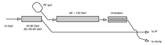
Figure 2: "Giga Z" configuration for polarised positron production.
