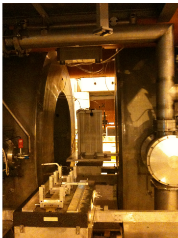
Figure 4.23: GRPC setup in the CERN SPS-H2 line magnetic field.
