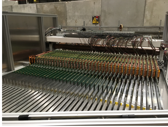
Figure 4.15: Fully integrated SiPM-on-tile AHCAL engineering prototype. (Courtesy DESY)
