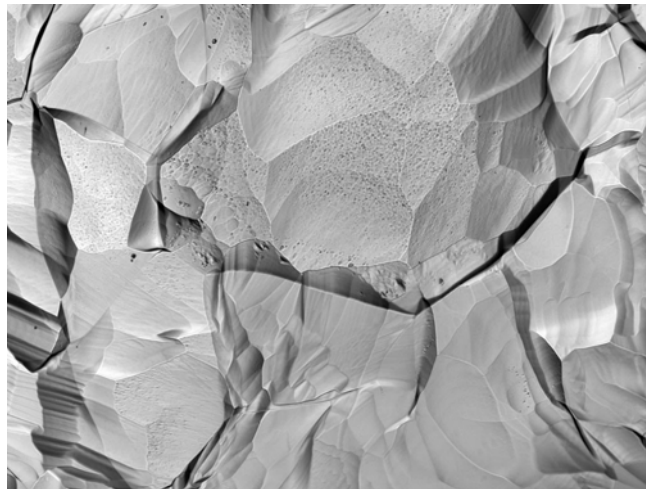
LEXT con-focal laser microscopy of a 100 \times 75 \mu\text{m}^2 region of polycrystalline Nb after chemical polishing with BCP 1:1:2. Courtesy of P. Lee (University of Wisconsin).
