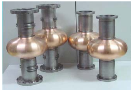
Some prototypes of Nb/Cu laminate cavities fabricated at DESY. Singer SRF-05
