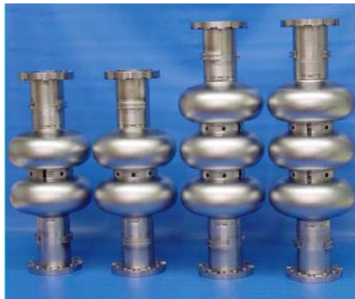
Singer-SRF05 – hydro-formed multi-cell cavities made from polycrystalline sheet material at DESY.
