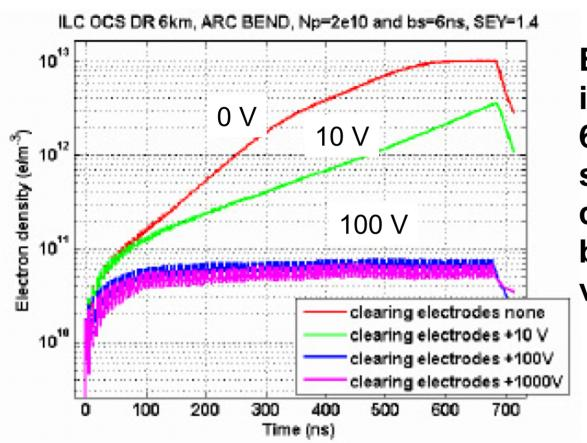
Electron cloud buildup in an arc bend of the 6.7 km ring and suppression effect of clearing electrodes biased at the indicated voltages.
